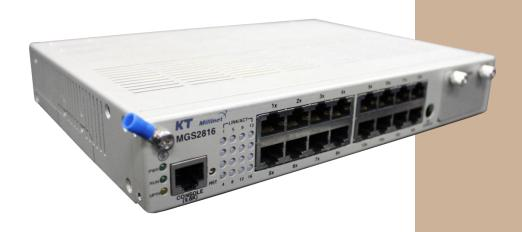
**OTS-G2016** is a Telco-Grade Gigabit Ethernet Switch suitable for IP based access network's concentrating equipment or solution for such construction as ETTH (Ethernet-to-the-home) and campus/internal building networking.
